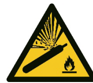
Pressure cylinder – remove in case of fire
